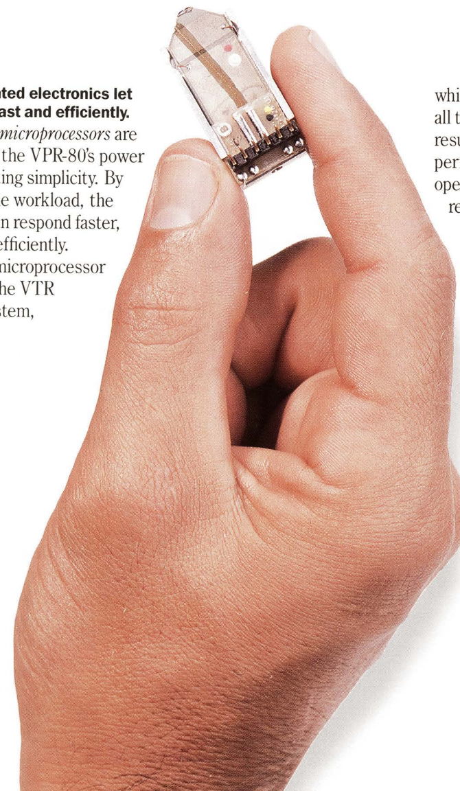
Both the Record and Playback functions are combined in a single, composite AST™ head. Both the AST and erase heads are easily removed and replaced with only a screwdriver.
